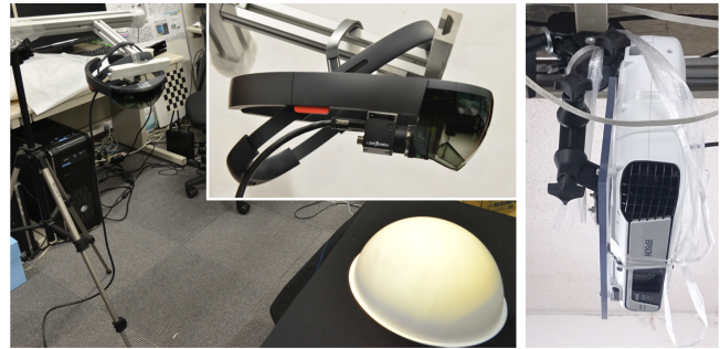
Figure 3: An overview of the hardware setup. (left) The SAR prop and HoloLens. The user-perspective camera installed behind the right optical element of the HoloLens. (right) The ceiling-mounted projector which displays a VI component on the prop.
