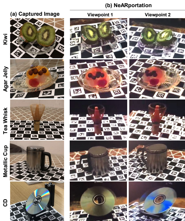
Figure 3: Qualitative performance overview of the NeARportation framework. (a) Captured images of real objects. (b) Real capture images of the reproduced appearances displayed on ELF-SR1, taken from two different viewpoints. Note that parallax artifacts appear in the images capturing the stereoscopic display because each image is taken directly with a monocular camera. This framework is interactive and is best viewed on video; thus, we urge readers to view our supplemental video.
